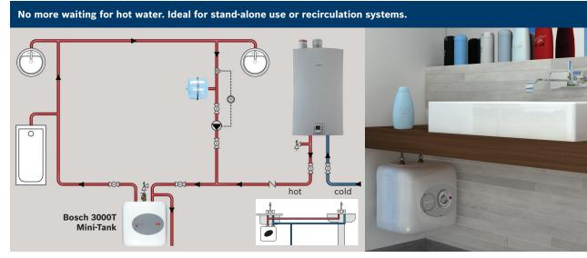
Relief valve is required; however it is not shown in above photo for clarity.
